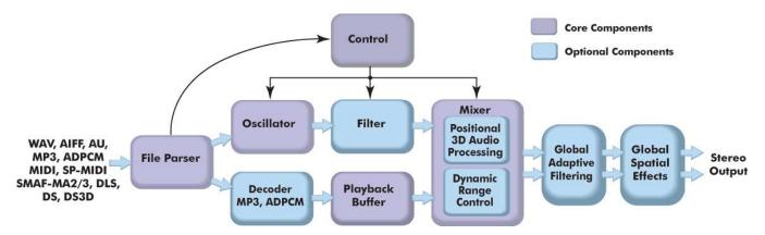
The flow diagram shows a representative configuration of **microQ** components. However, **microQ** architecture is a library of functional blocks that can easily be custom assembled into a multitude of combinations.
