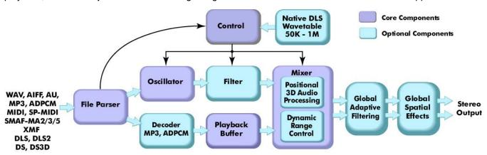
The flow diagram shows a representative configuration of **microQ** components. However, **microQ** architecture is a library of functional blocks that can easily be custom assembled into a multitude of combinations.
